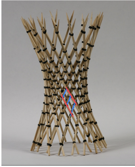
Figure 9: This shows a hyperboloid with circular symmetry that flexes into the plane around a circle, preserving lengths along the rulings. A typical ladder is shown in red and blue.
